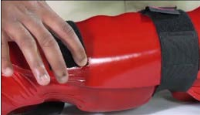
Finish smoothing glue along the seams to seal it.
